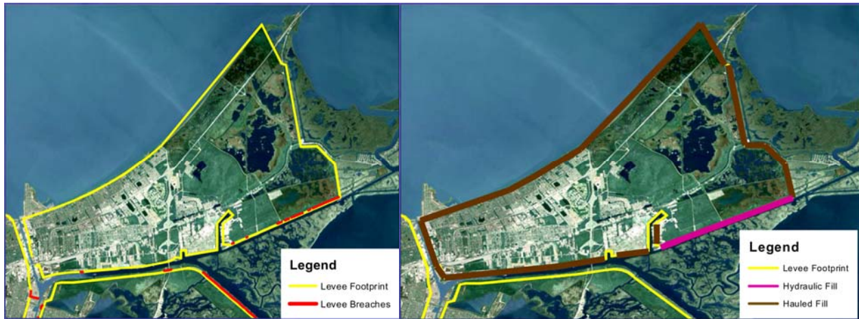
Figure 15. Correlation of levee breaching with type of levee materials for New Orleans East
